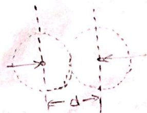
Diagram illustrating the collision diameter ( d ) as the distance between the centers of two molecules at the point of their closest approach.
